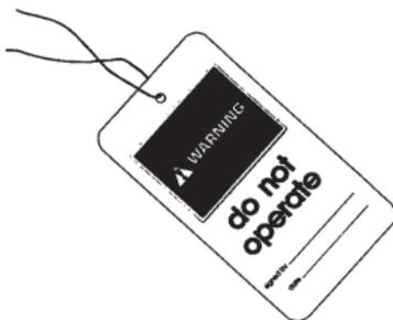
Attach a “**Do Not Operate**” warning tag or a similar warning tag to the start switch or to the controls before the engine is serviced or before the engine is repaired. These warning tags (Special Instruction, SEHS7332) are available from your Caterpillar dealer. Attach the warning tags to the engine and to each operator control station. When it is appropriate, disconnect the starting controls.
